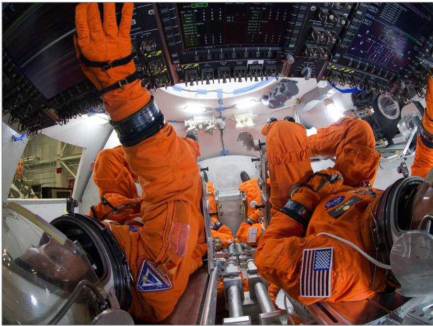
Figure 1 | Spacesuited engineers demonstrate how four crew members would be arranged for launch inside the Orion spacecraft, using a mockup of the vehicle at Johnson Space Center. (Photo credit: NASA/Robert Markowitz.)
