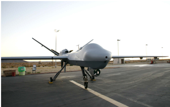
Figure 1 | Due Regard Radar is aimed at enabling users to operate the Predator B unmanned aerial vehicle independently in international airspace without the need for land-based, sea-based, or off-board airborne airspace surveillance. Photo courtesy of General Atomics.
