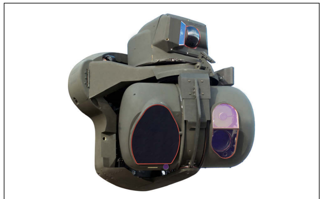
Figure 2 | The Modernized Target Acquisition Designation Sight/Pilot Night Vision Sensor (M-TADS/PNVS) system is the advanced electro-optical fire control system used by AH-64D/E Apache helicopter pilots. Photo courtesy of Lockheed Martin.
