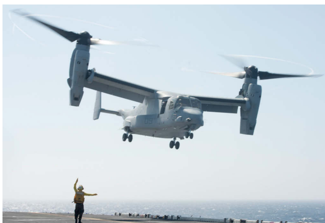
Figure 3 | The V-22 Osprey is a joint-service, multimission combat aircraft combining the mobility of a helicopter with the long-range, high-speed cruise performance of a turboprop. Photo courtesy of U.S. Navy.
